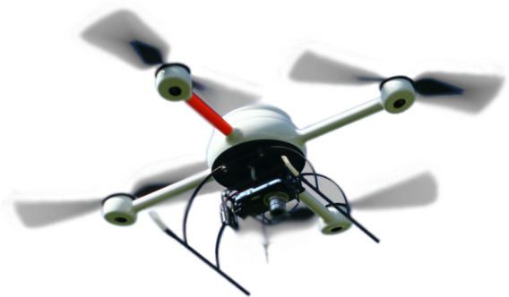
Figure 1: Small-scale microdrone with an attached camera.
